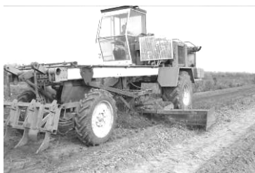
Fig.2. Universal self-propelled soil arrangement machine USM-5
