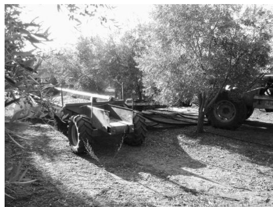
Figure 6. Rolling canvas for high density olive orchards
