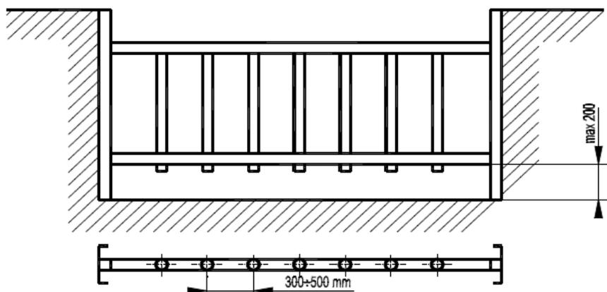
Fig.1. Positioning of the electrical repeller ELZA2 copper electrodes.
