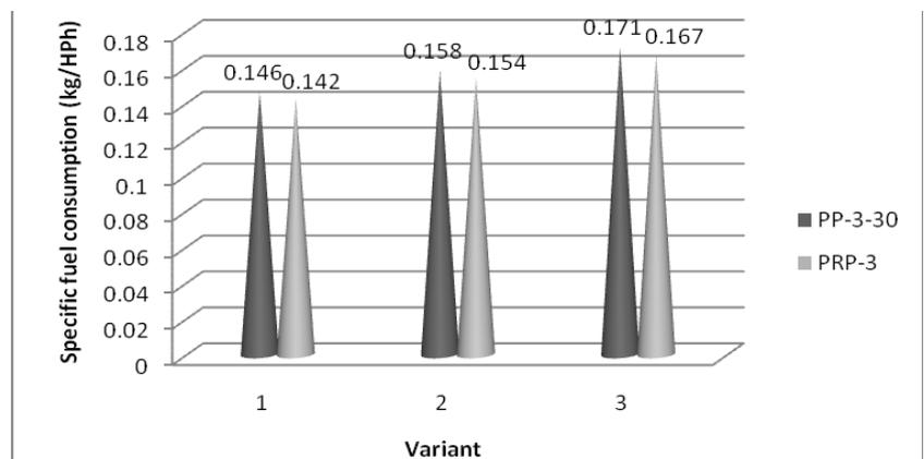
**Graph 2. Variation of fuel specific consumption function of soil type ( $v_2 = 4.61 \text{ km h}^{-1}$ )**
