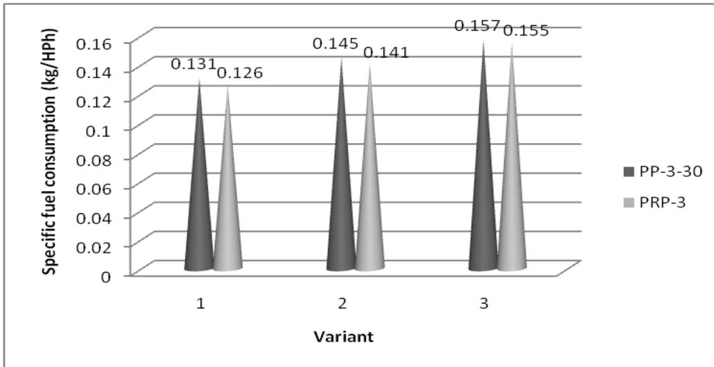
**Graph 4. Variation of fuel specific consumption function of soil type ( $v_4 = 4.98 \text{ km h}^{-1}$ )**
