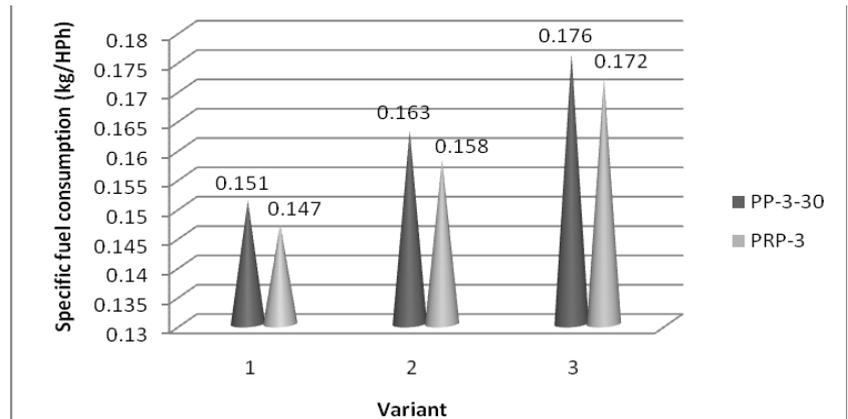
**Graph 1. Variation of fuel specific consumption function of soil type ( $v_1 = 4.48 \text{ km h}^{-1}$ )**
