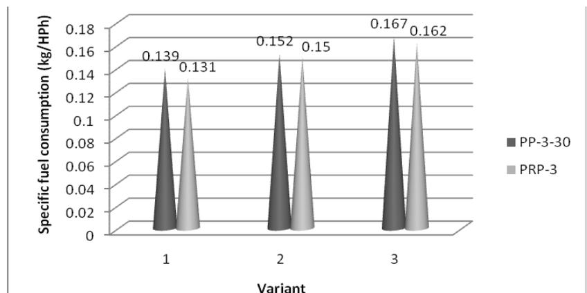
**Graph 3. Variation of fuel specific consumption function of soil type ( $v_3 = 4.85 \text{ km h}^{-1}$ )**
